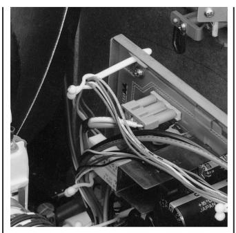
This connector can be connected to headers having 2.36mm diameter pins. Since the pitch between circuits is large, 8.0mm, this connector is ideally suited for the power supply circuits of TVs, stereo systems and VCRs.
