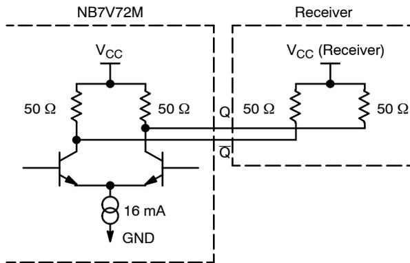
Figure 11. Typical CML Output Structure and Termination
