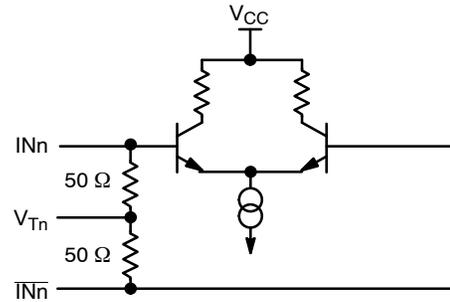
**Figure 4. Input Structure**
