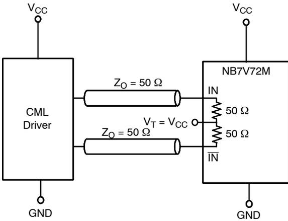
Figure 15. Standard 50  $\Omega$  Load CML Interface
