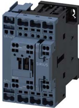
Contactor, AC-1, 35 A/400 V/40 °C, S0, 4-pole, 24 V AC/50 Hz, 1 NO+1 NC, Spring-type terminal
