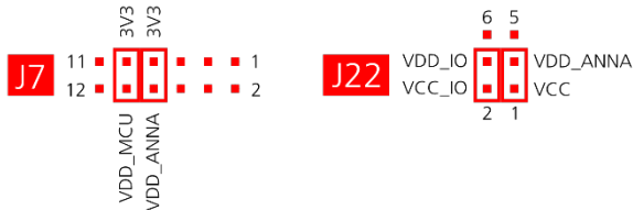
Figure 8: Jumper positions for default power configuration
