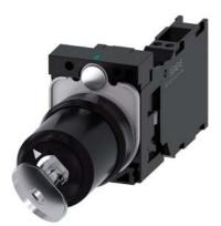
key-operated switch Siemens, 22 mm, round, plastic, lock number SSG10, with 2 keys, 2 switch positions O-I, latching, 10:30h/13:30h, key removal O+I, with holder, 1 NO+1 NC, spring-loaded terminal, with laser labeling, upper case and lower case, always upper case at beginning of line
