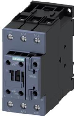
power contactor, AC-3e/AC-3, 51 A, 22 kW / 400 V, 3-pole, 24 V DC, 0.8-1.2\* Us, with integrated varistor, auxiliary contacts: 1 NO + 1 NC, screw terminal, size: S2, suitable for PLC outputs
