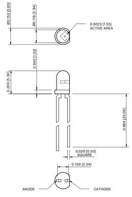
Note: Lead soldering temperature (5mm from body) 260°C for 5 sec.
