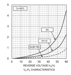
REVERSE POWER DISSIPATION:P<sub>R</sub>(W)
