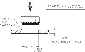
INSTALLATION FORCES CAN VARY FROM 1 TO 5 TONS.
