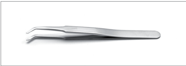
SM112.SA Tips: positioning 5mm monolithic chip capacitors at 60°, grooved. OAL: 120mm
