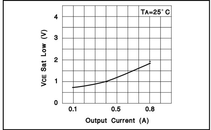
Figure 3: Typical Sink Saturation Voltage vs Output Current
