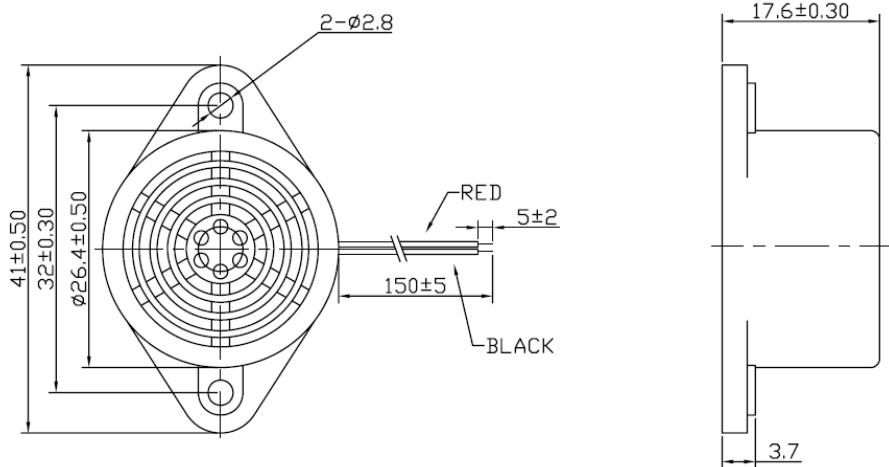
Dimensions Unit: mm Tolerance:  $\pm 0.5\text{mm}$
