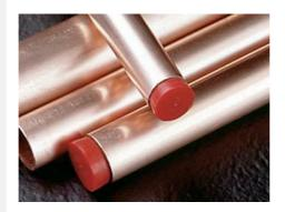
K Series copper tubing plugs are especially suitable for general purpose, Type K copper tubing, SAE Standard J-528. This series is designed for applications where the outside diameter of the closure should not exceed the outside diameter of the tubing. Flanges fit flush with outer walls of tubing, providing positive protection against moisture and dirt.
