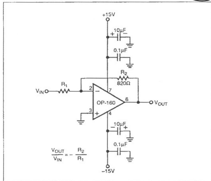
FIGURE 21: The OP-160 as an inverting amplifier.
