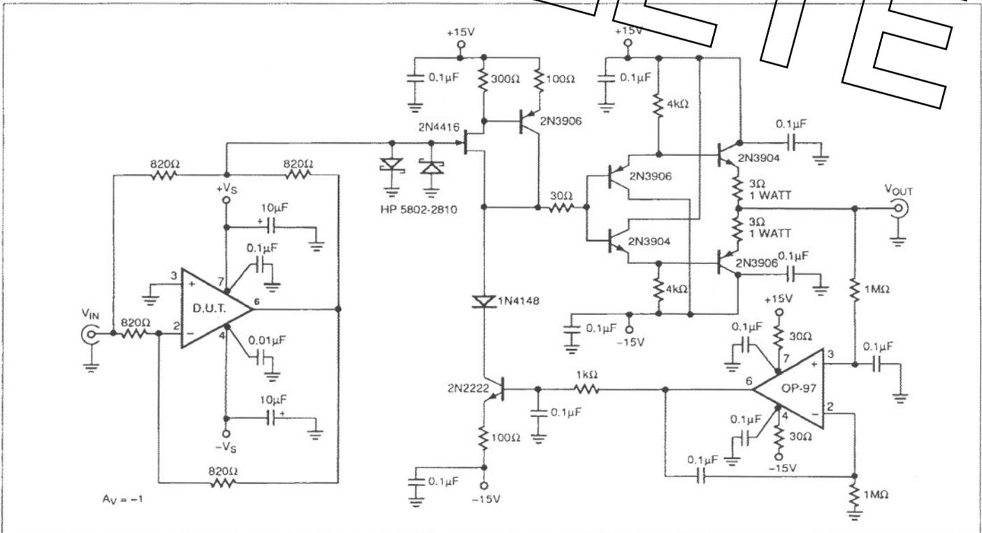
**FIGURE 10:** High-Speed Settling Time Fixture (for 0.1 and 0.01%)
