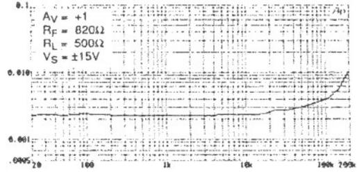
**INPUT VOLTAGE NOISE DENSITY vs FREQUENCY**
