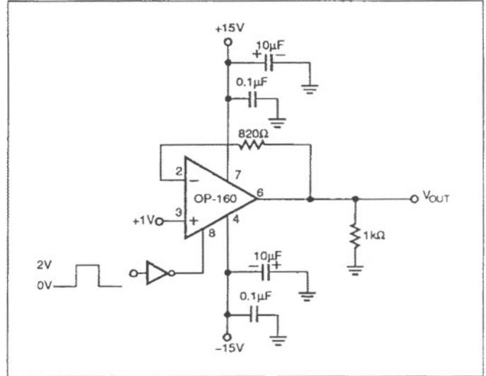
FIGURE 16:  $\overline{\text{DISABLE}}$  Turn-On/Turn-Off Test Circuit
