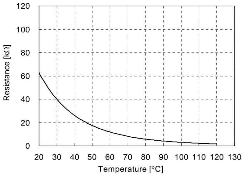
**Figure 5. R-T Curve of the Built-In Thermistor**
