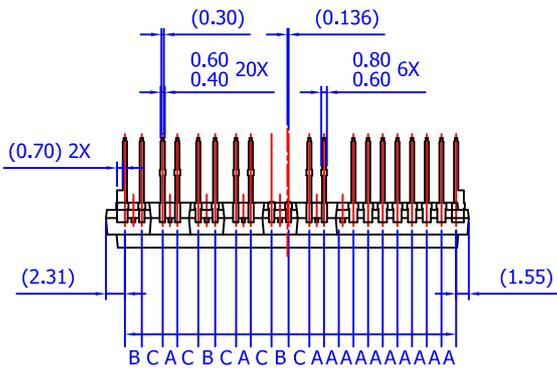
LEAD PITCH (TOLERANCE : ±0.30)
