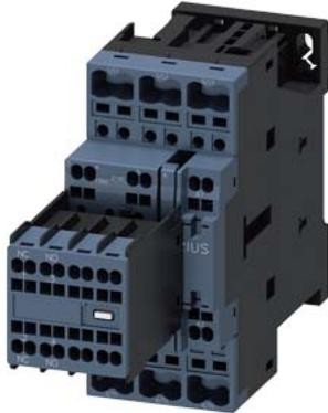
power contactor, AC-3e/AC-3, 17 A, 7.5 kW / 400 V, 3-pole, 230 V AC, 50/60 Hz, auxiliary contacts: 2 NO + 2 NC, spring-loaded terminal, size: S0, removable auxiliary switch
