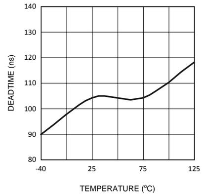
Figure 8. Dead Time vs Temperature R<sub>SET</sub> = 29.5 kΩ
