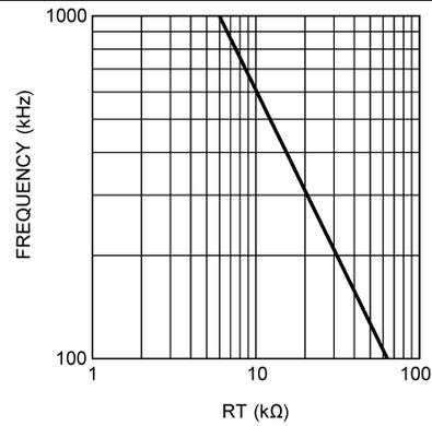
Figure 4. Oscillator Frequency vs  $R_T$
