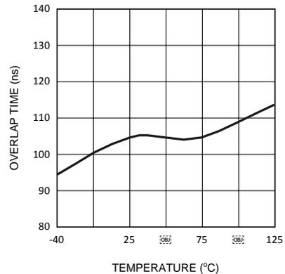
Figure 6. Overlap Time vs Temperature  $R_{SET} = 38 \text{ k}\Omega$
