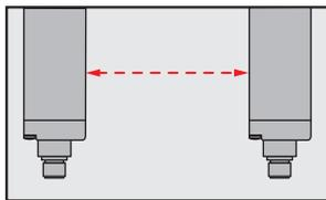
The light grid communicates via the light beams. A cable is not necessary for the optical synchronisation.
