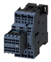
power contactor, AC-3e/AC-3, 12 A, 5.5 kW / 400 V, 3-pole, 24 V DC, auxiliary contacts: 2 NO + 2 NC, spring-loaded terminal, size: S0, removable auxiliary switch
