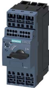
Circuit breaker size S0 for motor protection, CLASS 10 A-release 0.45...0.63 A N-release 8.2 A Spring-type terminal Standard switching capacity with transverse auxiliary switches 1 NO+1 NC
