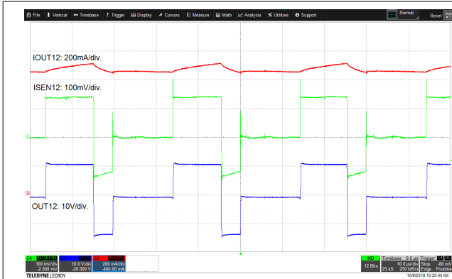
Figure 8-11. Zoomed Waveform Showing Current Regulation
