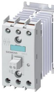
Solid-state contactor 3-phase 3RF2 AC 51 / 10 A / 40 °C 48-600 V / 230 V AC 2-phase controlled screw terminal Blocking voltage 1200 V
