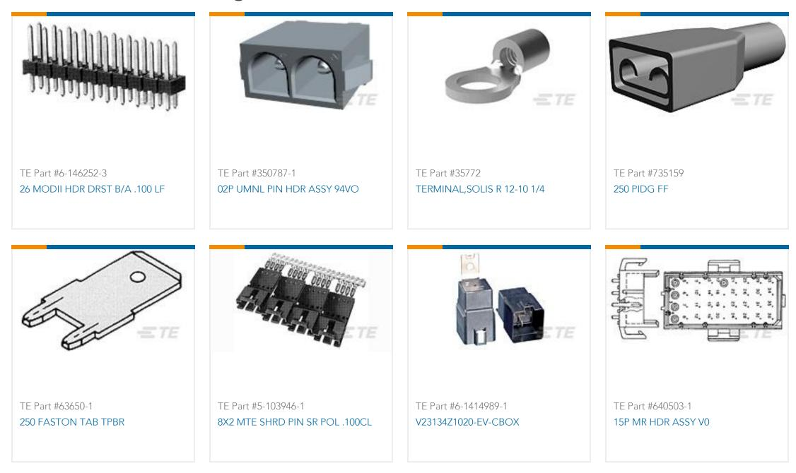
Closed Ring Tongue Terminal, 12 – 10 AWG, 5/16 / M8 Stud Size, 8.3 mm [.327 in] Stud Diameter, Closed Barrel, Straight, Tin, Uninsulated
