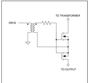
Figure 1. Sampling circuit with two FETs.
