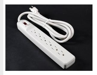
Basic surge protection. Six outlets, lighted switch, impact-resistant putty white polymetric housing, 15A. 6' [1.8m] 14/3 SJT putty white cord with NEMA5-15 plug. Maximum surge current 6500 Amps. 11 3/4" x 2 1/4" x 1 1/2 [298mm x 57mm x 38mm]. Keyhole mounting.
