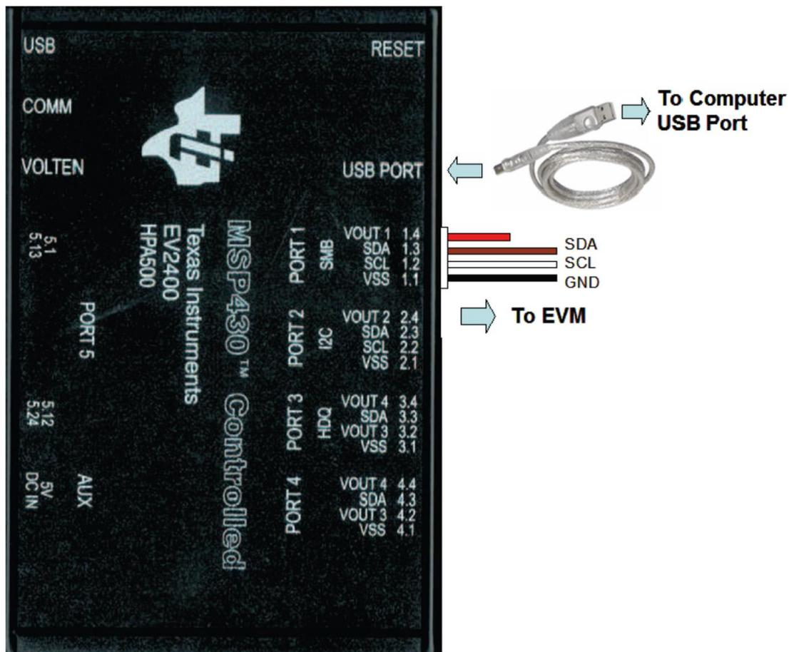
The picture shows the SMBus version EVM connection. If using the BQ25713EVM-017, move the connector to the I<sup>2</sup>C port.
