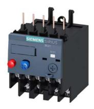
Overload relay 2.8...4.0 A Thermal For motor protection Size S00, Class 10 Contactor mounting Main circuit: Ring cable lug Auxiliary circuit: ring cable lug Manual-Automatic-Reset
