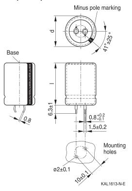
Snap-in terminals, length (6.3 ±1) mm. Also available in a shorter version with a length of (4.5 - 1) mm. Insulation is marked with "PET" on the sleeve. Safety vent on the base.
