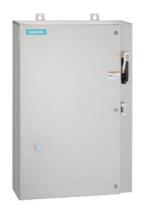
Non-reversing motor starter, Size 0, Three phase full voltage, Solid-state overload relay, OLRelay amp range 0.75-3.4a, 110V 50HZ / 120V 60HZ coil, Combination type, 30Amp fusible disconnect 30 Amp /600V fuse clip, Encl NEMA type 4X 316 S-steel Water/dust tight noncorrosive, Extra-wide enclosure
