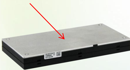
Figure 42: Thermal test point
