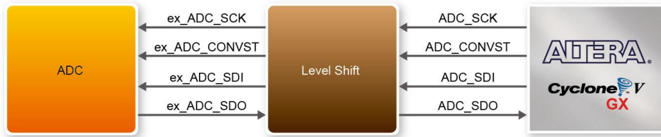
Figure 6-23 Hardware connection between FPGA and ADC
