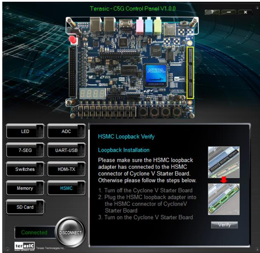
Figure 2-12 HSMC loopback verification test performed under Control Panel
