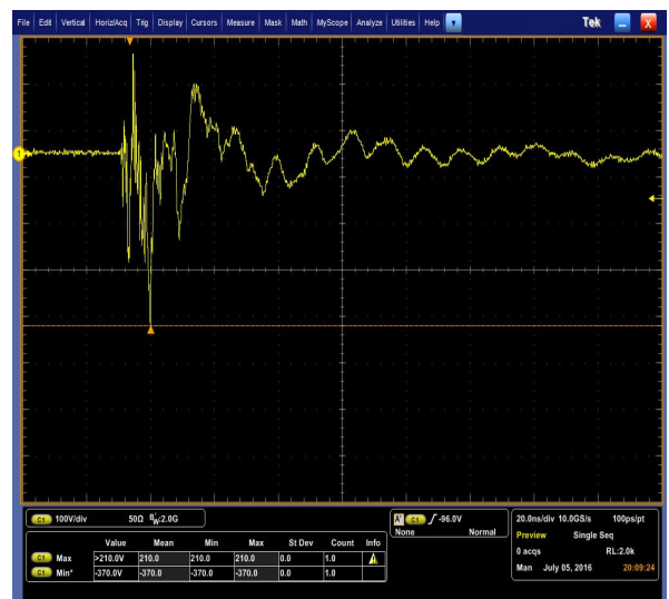
Figure 2. ESD Clamping Voltage Screenshot Negative 8 kV Contact per IEC61000-4-2
