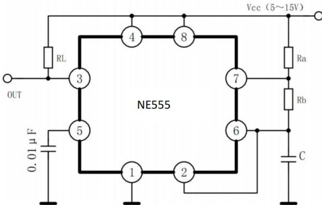
振荡周期:  $T=0.693 (R_A+2R_B) C$     占空比:  $D=R_B / (R_A+2R_B)$
